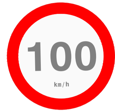
100kph REPEATER SIGN (RUS 040) 450Ømm TO BE REMOVED & RELOCATED
