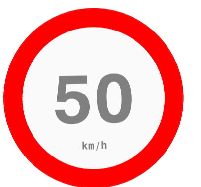
50kph REPEATER SIGN (RUS 043) 450Ømm TO BE REMOVED & RELOCATED
